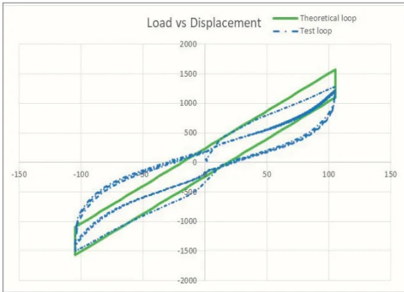
Fig. 13: Force-displacement diagram of EQS23600 (LHS) – comparison with theoretical loop
