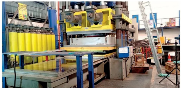
Fig. 7: Bearing testing in Dynamic Testing Machine
