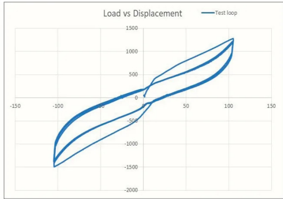
Fig. 12: Force-displacement diagram of EQS23600 (LHS) – test for seismic movement
